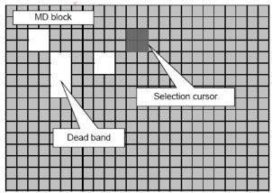
The dead band setting function enables the on-screen cursor to be moved in response to the input of operating Left, Right, Up and Down and whether to set the sensing band or dead band for the specified blocks to be selected by the Enter operation input.
